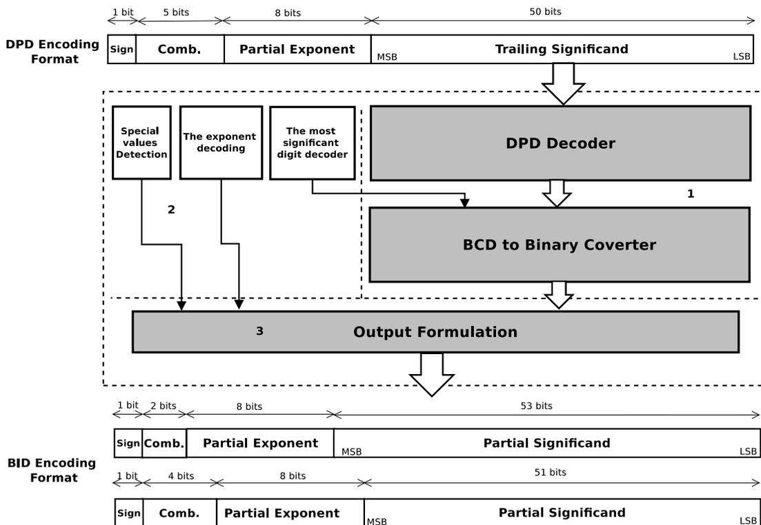
Figure 3.6: DPD to BID converter (64 bits) block diagram
