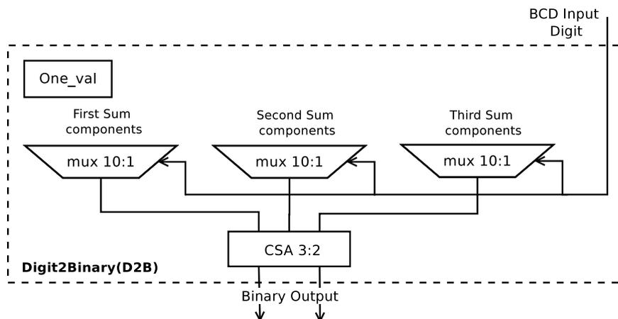
Figure 3.8: Digit to Binary block architecture
