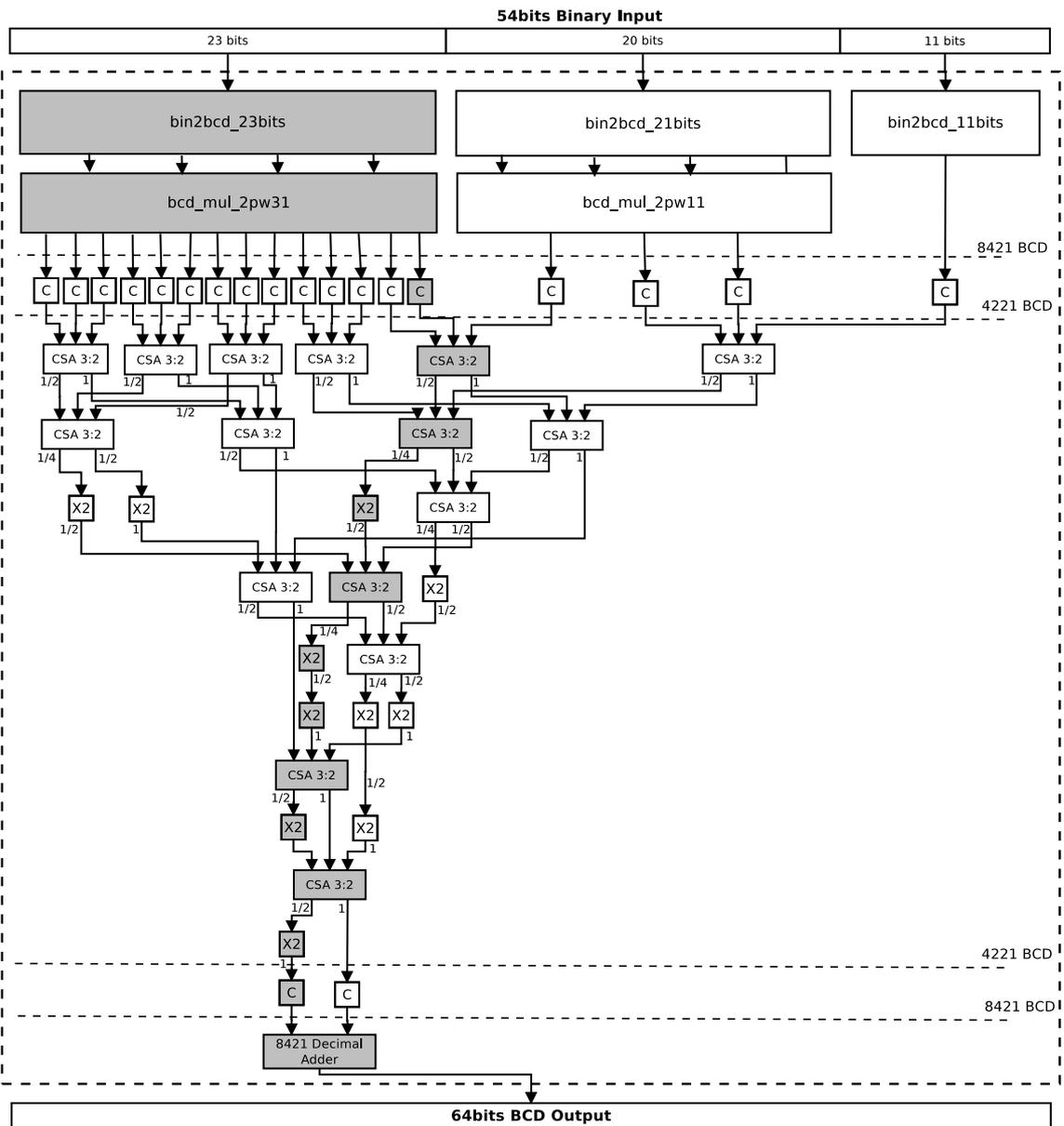
Figure 3.15: 54bits Binary to BCD Converter – The first design
