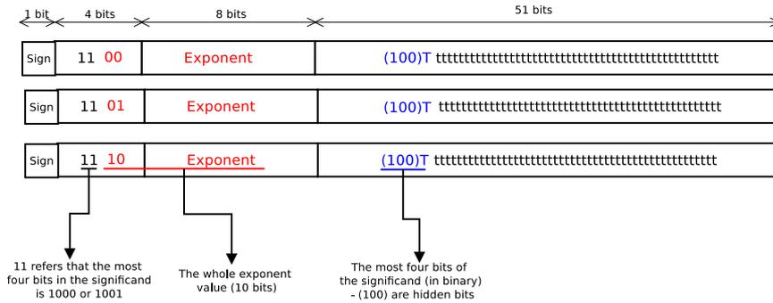
Figure 1.5: Binary Integer Decimal Encoding format for the most significant digit from 8 – 9, 64 bits
