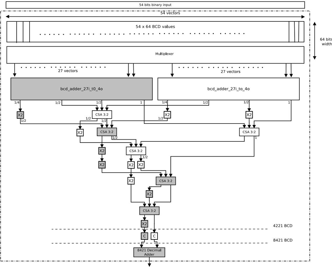
Figure 3.18: 54bits Binary to BCD Converter – The third design
