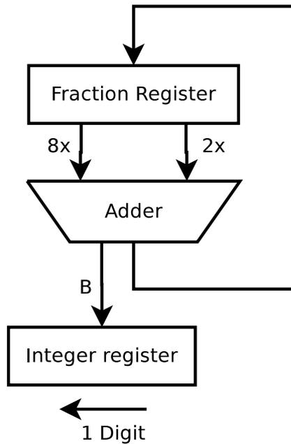
Figure 1.14: The sequential Binary to BCD converter - 1 Digit per cycle
