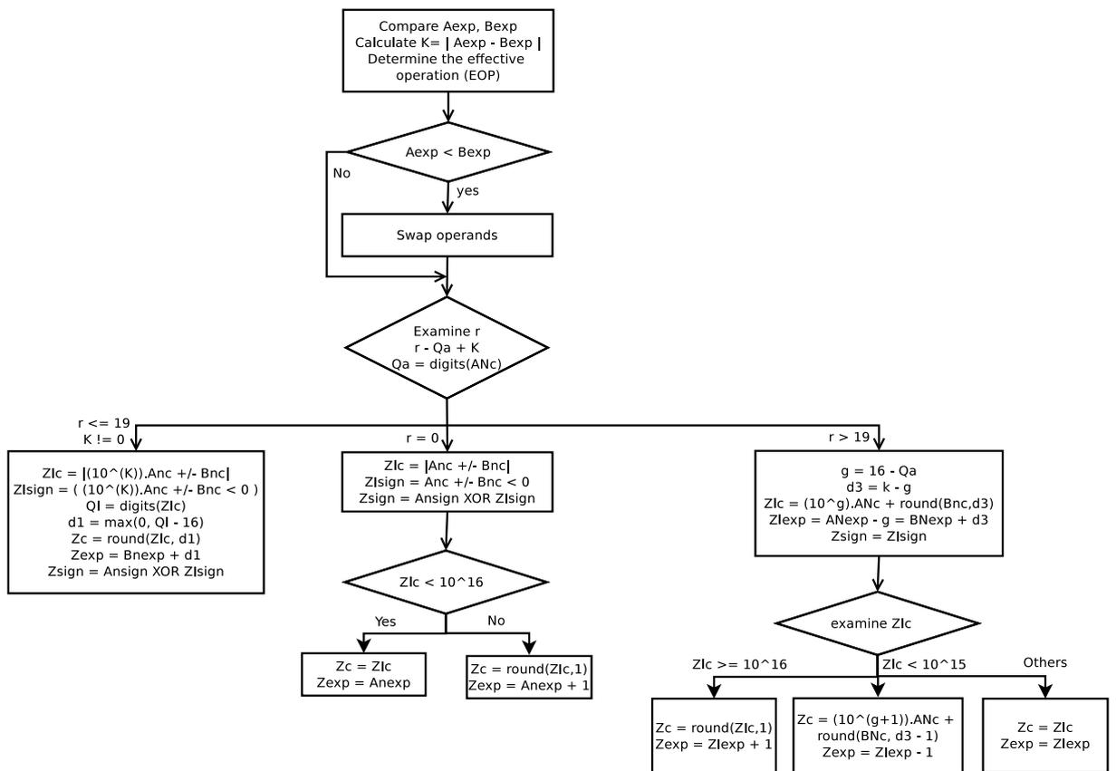
Figure 3.21: The BID Addition/Subtraction Algorithm Flowchart
