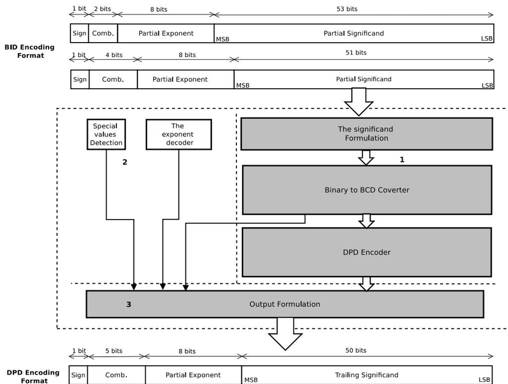
Figure 3.14: Binary Integer Decimal to Densely Packed Decimal Converter block diagram - 64 bits
