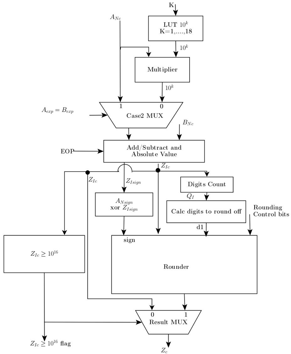
Figure 3.20: Direct Hardware For Cases 1 and 2
