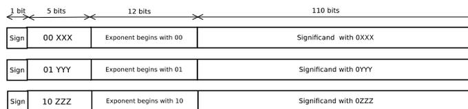
Figure 3.12: DPD128 Encoding format for most significant digit from 0 – 7
