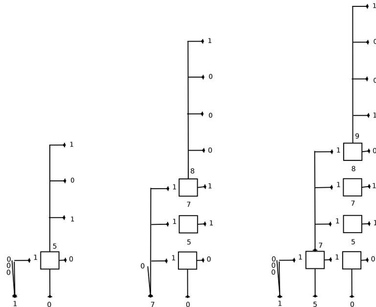
Figure 1.18: An example for binary to decimal conversion algorithm in [32] for integer numbers
