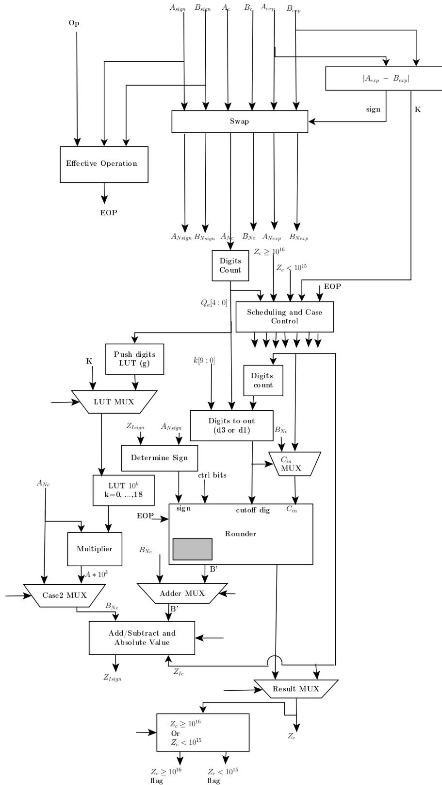
Figure 3.28: Adder HW Design Combined with Case 1, 2 and 3
