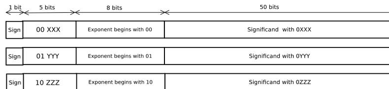
Figure 1.8: DPD64 Encoding format for the most significant digit from 0 – 7
