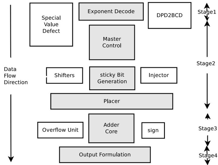
Figure 3.4: SilMinds DFP Adder architecture
