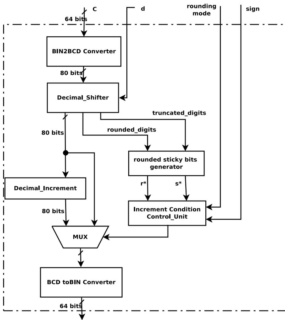
Figure 3.27: The Proposed Rounder Block Diagram
