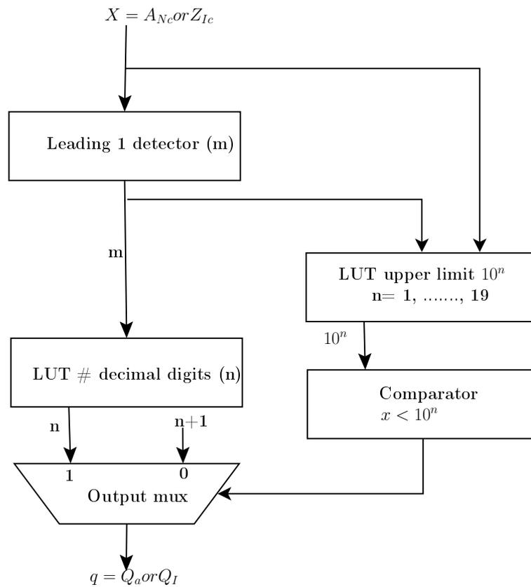
Figure 3.23: Decimal Digit Counter Block Diagram
