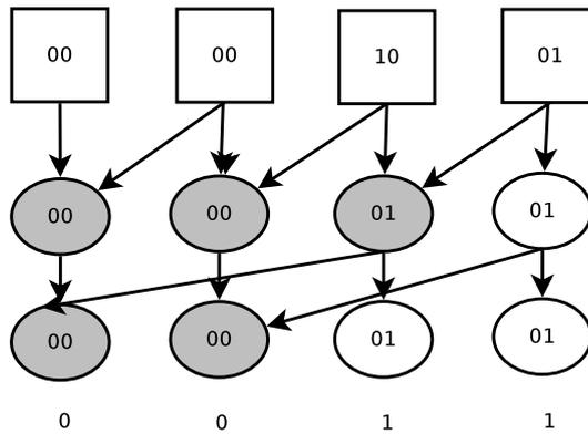
Figure 3.24: An example of decimal incrementer which uses kogge-stone tree
