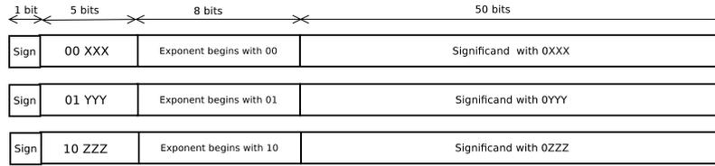
Figure 3.10: DPD64 Encoding format for the most significant digit from 0 – 7
