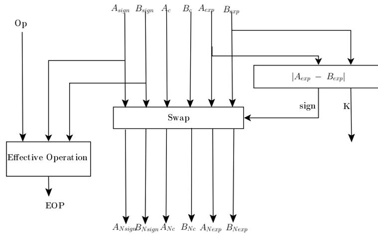
Figure 3.19: Hardware For Algorithm Step 1
