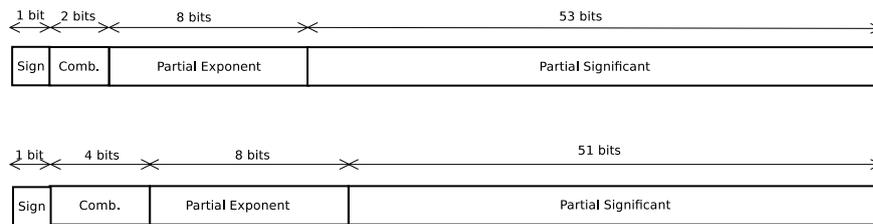
Figure 1.2: Binary Integer Decimal Encoding - 64 bits
