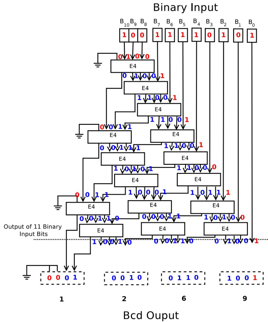
Figure 1.12: 11 Binary bits to BCD decoding tree with E4 decoders numerical example
