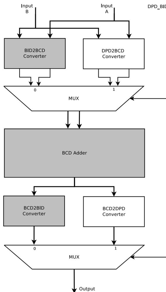
Figure 3.1: Generic architecture of our proposed adder design
