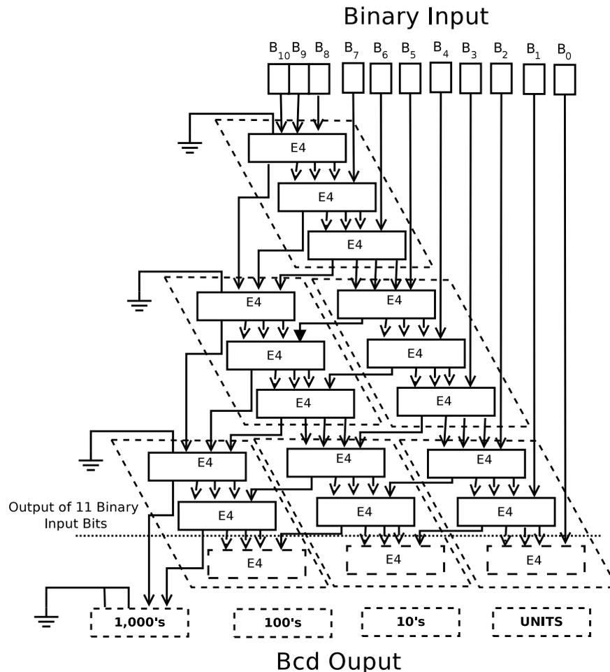
Figure 1.11: 11 Binary bits to BCD decoding tree with E4 decoders, the dotted outlines represent E6 decoders
