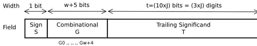
Figure 1.1: Decimal Floating-Point Interchange Format
