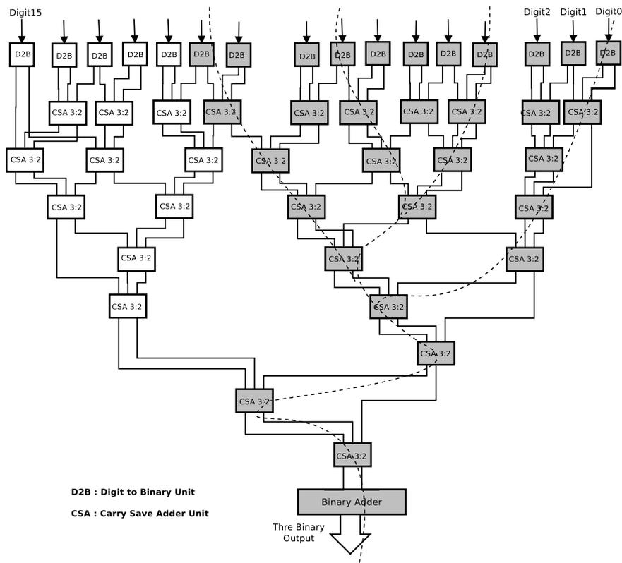
Figure 3.9: BCD to Binary Adder tree - 64 BCD input bits
