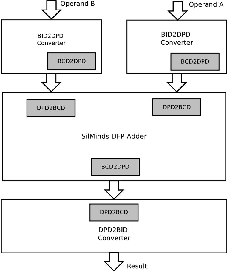
Figure 3.2: Our Proposed DFP Adder Architecture
