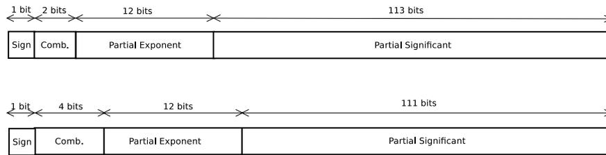
Figure 1.3: Binary Integer Decimal encoding - 128 bits
