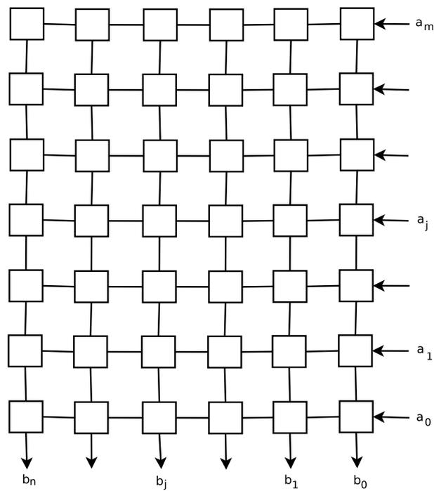
Figure 1.17: Two-dimensional iterative array for conversion of an integer from a radix  $p$  to a radix  $q$  number system
