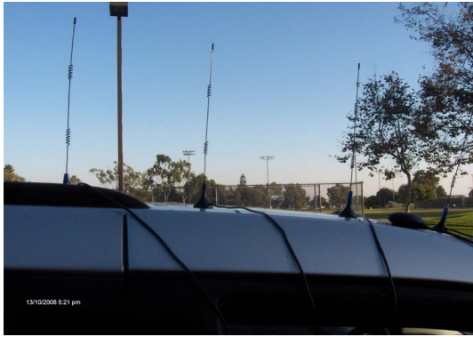
Fig. 5. The outdoor receiver: tall antennas on top of a van
