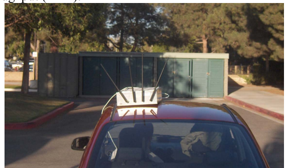
Fig. 4. The outdoor transmitter: MWLAN board on top of a car
