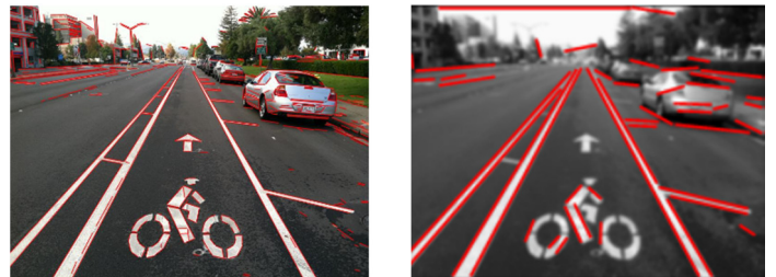
Fig 3 The effect of using the Gaussian Pyramid on the number of lines detected by line detection algorithm. The original image to the left and the image after applying 3-level Gaussian Pyramid to the right
