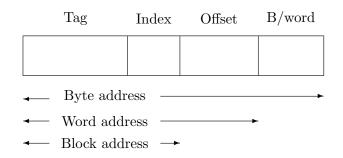
Let us try to find the size of a cache with 9 bits index in a machine having 32 bits for its addresses assuming that the word is four bytes and the block is eight words. Why eight words in a block?
