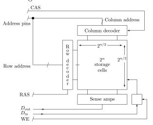
The DRAM controller multiplexes the address and provides the RAS and CAS to the chip. To get a faster access, we use
