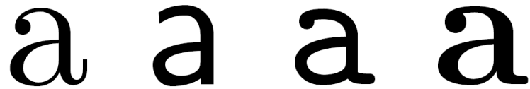
Figure 3.6: Four different lowercase letter ‘a’ forms generated by a single description program. From left to right: roman, sans serif, typewriter, and bold.
