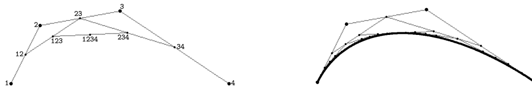
Figure 4.6: A Bézier curve. Points 2 and 3 are the control points of the curve, and are calculated by METAFONT from the tangential direction of the curve at the ending points.
