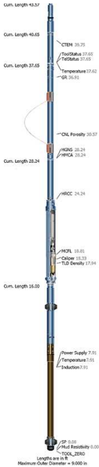
Figure 1-2 GR - Density -Litho logy, and Induction Resistivity Tool String
