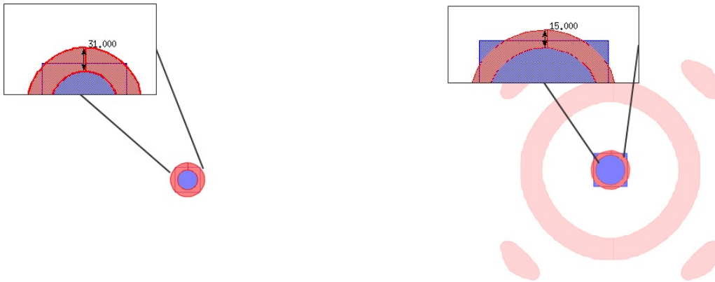
Figure 3.9: Impact of inserting SRAF for isolated contact across where the left hand side is the line width deviation of the contour without SRAFs and the right hand side is the response for with SRAFs. Left hand side shows CD [1].
